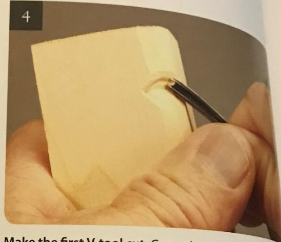
Make the first V-tool cut. Carve the upper eyelid. Carve along the inside crease of the top eyelid with a sharp \frac{1}{8} " V-tool. This separates the upper eyelid from the eye socket.
