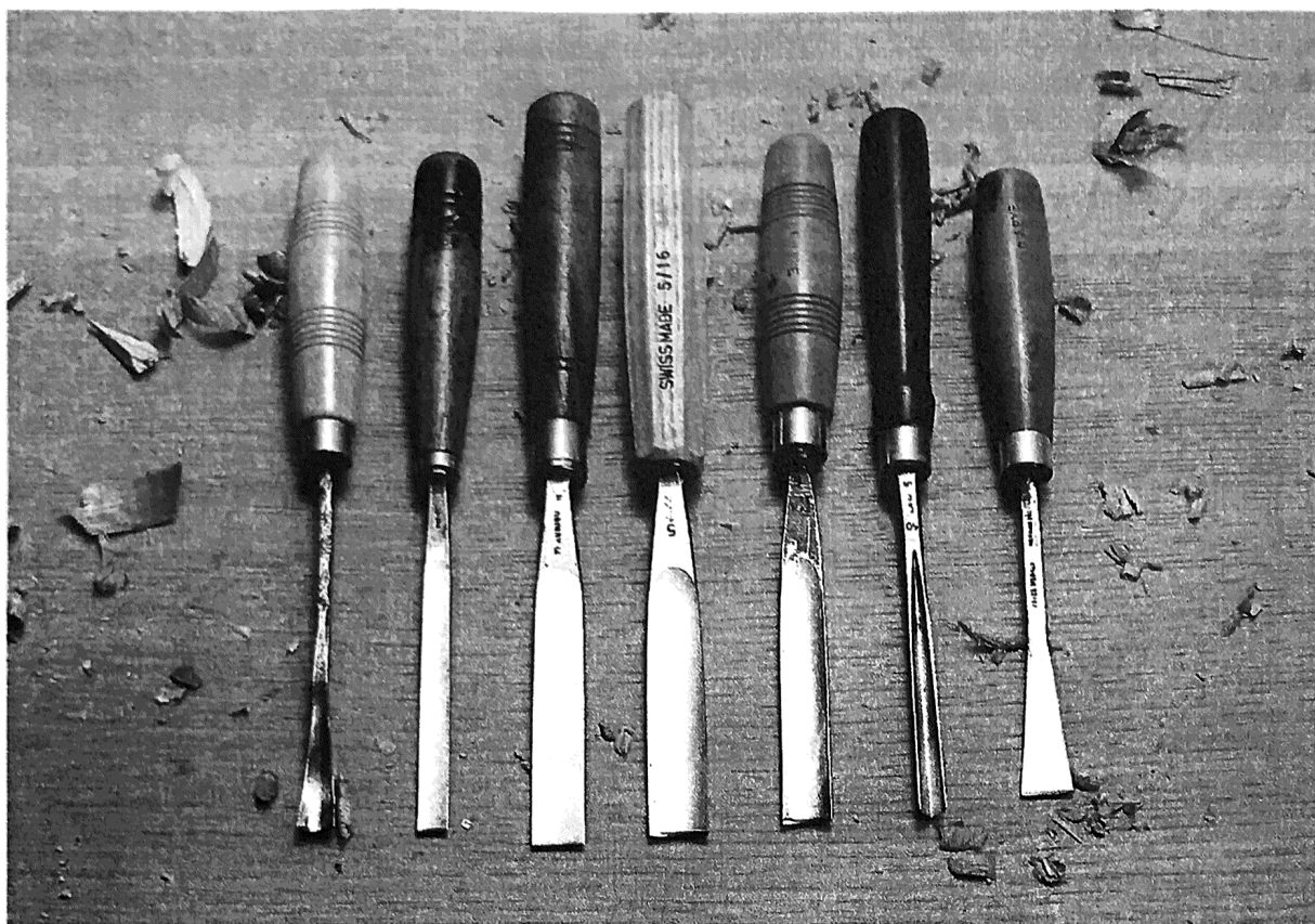
Fig 7.8 Lining up the tools in use keeps their edges from knocking against each other and makes them easier to recognize
