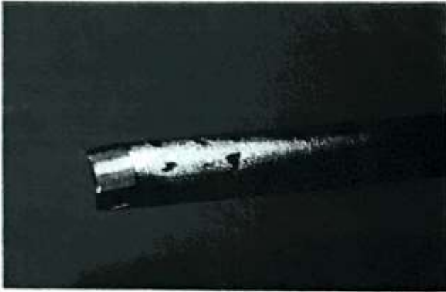
Fig 12.60 The 'candle' effect: a final rim of polished metal towards the edge. The duller, honed surface creeps towards it as the bevel is flattened. The corners and straightness of the cutting edge will need checking over too
