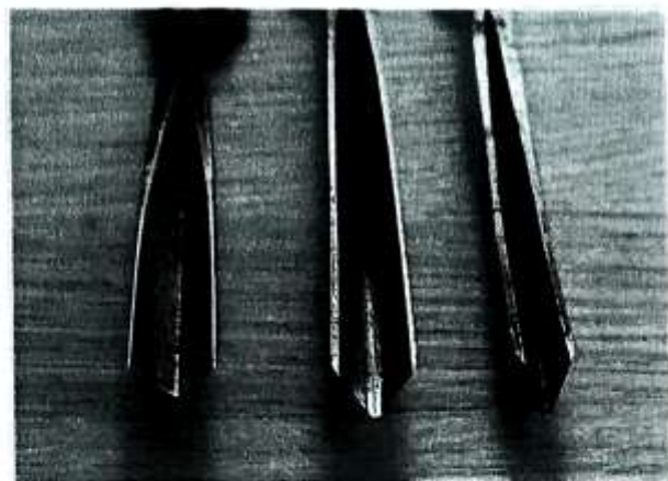
Fig 12.32 The three different V-tool angles will need corresponding angles on the slipstones
