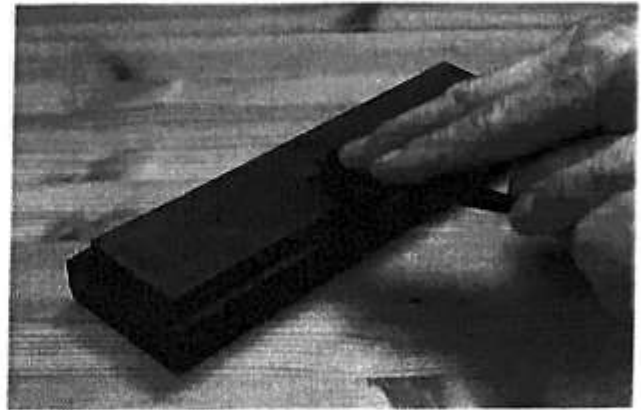
Fig 12.39 Rounding over the keel of the V-tool by careful rubbing on the benchstone. As always, present the bevel flat and keep checking the edge by its line of light
