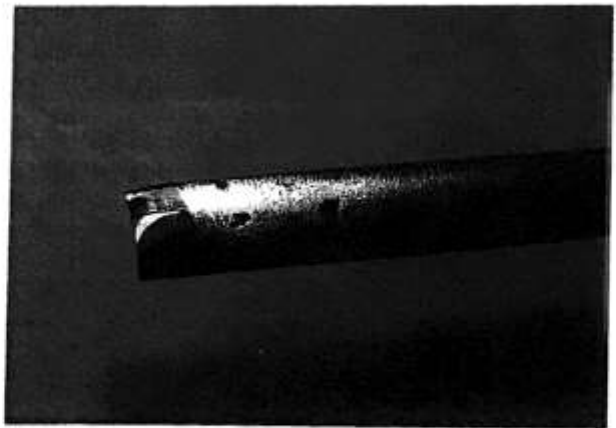
Fig 12.59 The curved reflection on this highly polished surface is a clue that the bevel has become rounded
