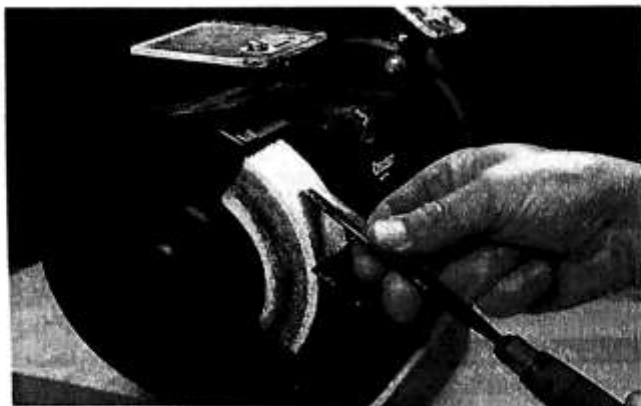
Fig 12.4 In-line presentation, with fingers on toolrest
