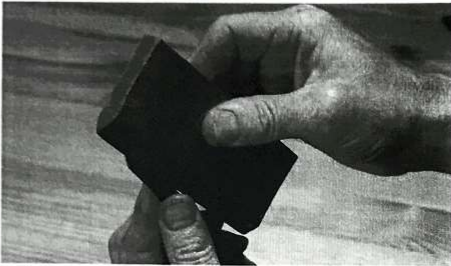
Fig 12.41 A specially made V-tool slipstrop. Keep your fingers clear
