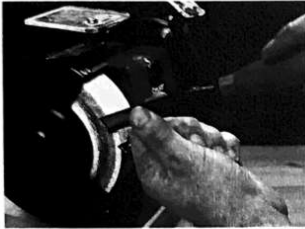
Fig 12.6 Touching the carving tool to the side of the grinding wheel; only the lightest touch is permissible
