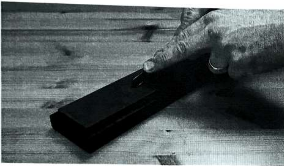
Fig 12.35 Treat one side of the V-tool like a chisel . . .
