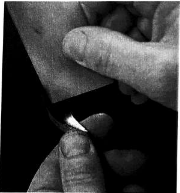
Fig 12.50 Using a slip to remove the burr on the inside edge of a frontbent gouge
