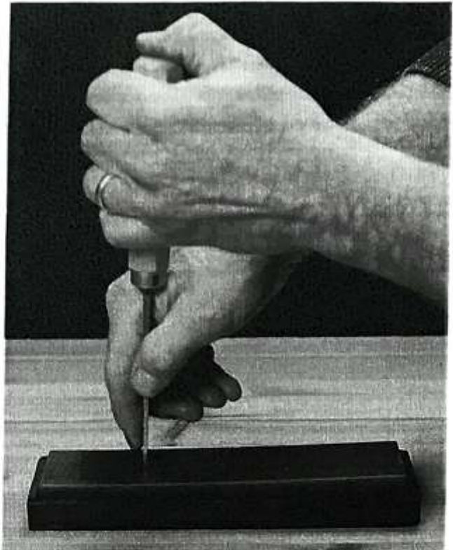
Fig 12.11 Cleaning the edge of a carving tool involves offering it in a perpendicular position and pulling it along a flat benchstone. This is necessary each time you move to a finer stone, refining the edge from the coarser grit of the previous one
