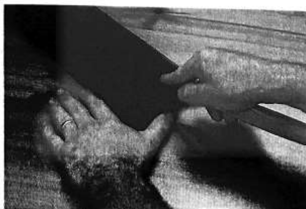
Fig 12.23 The hand that steadies the strop must be kept out of the way of the returning cutting edge
