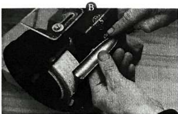
Fig 12.8 Flatten the bevel by offering it square-on to the rotation. Do this lightly and make sure your hand is supported by the toolrest. If preferred, this method can be used for all the bevel shaping
