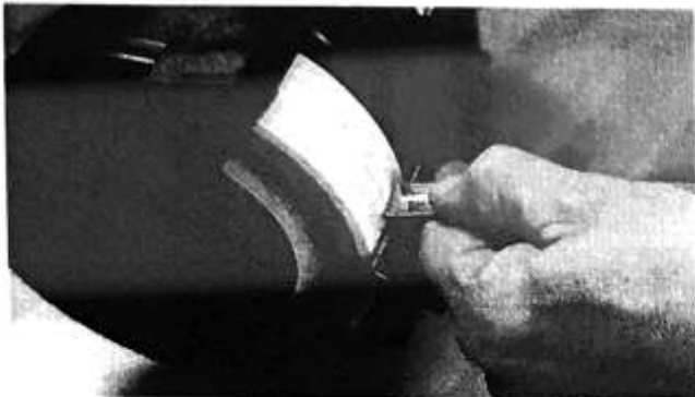
Fig 12.3 Perpendicular presentation (for clarity the grinder's perspex guards are swung up)
