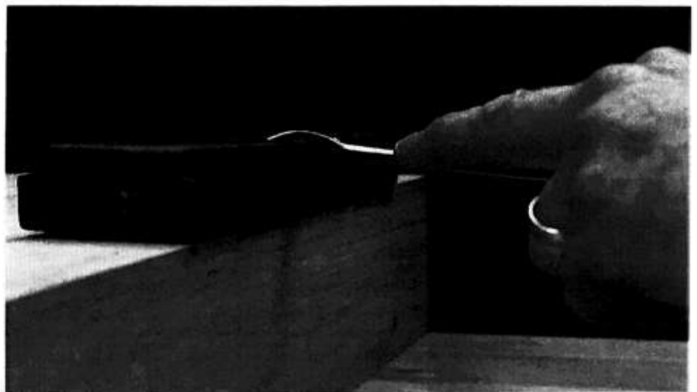
Fig 12.56 Slipstones are used with the benchstone to sharpen a backbent gouge
